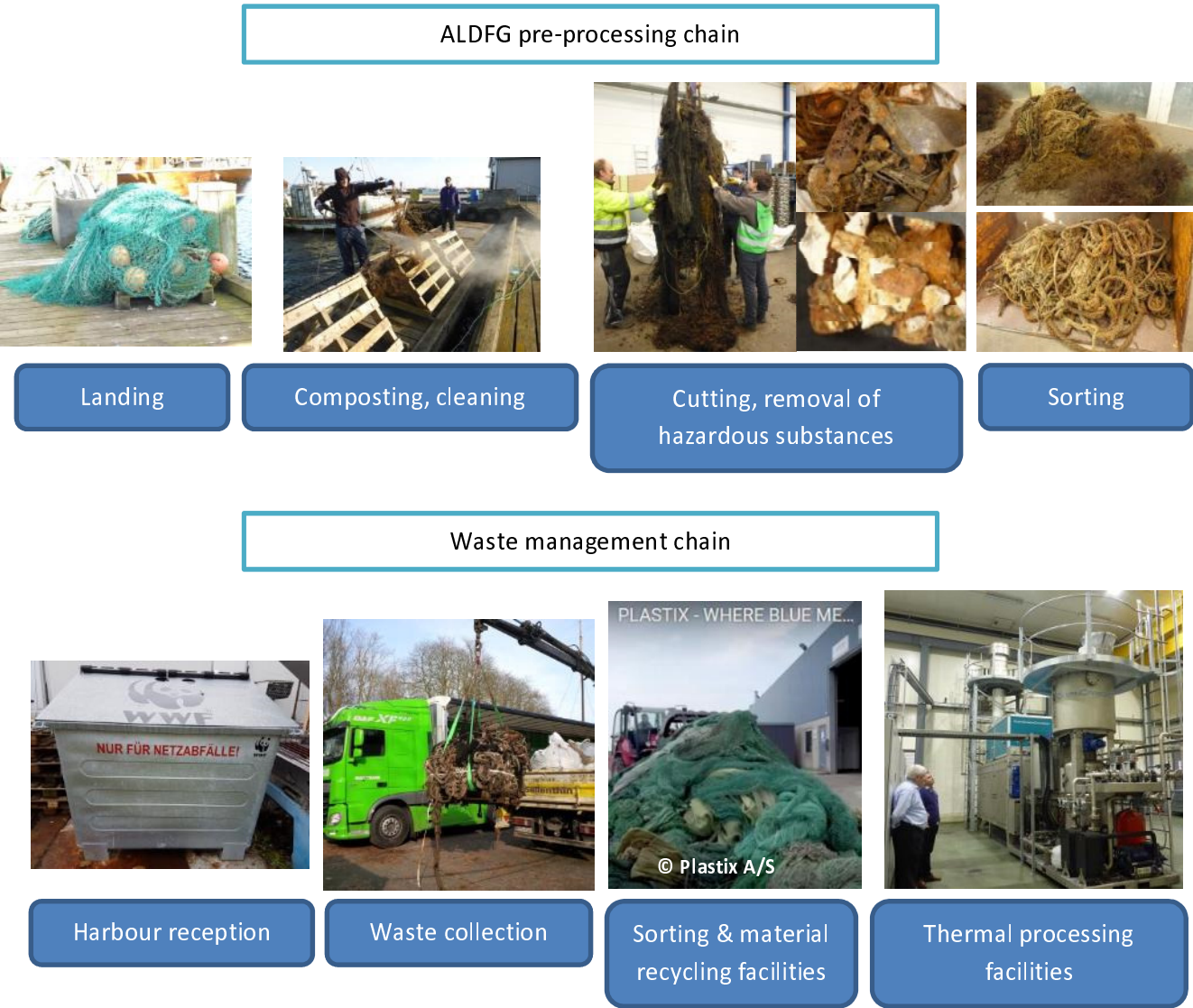
Fig. 13 From harbour landing to waste management. Top: Pre-processing chain in preparation for waste management. Bottom: Waste management chain from harbour reception to material recycling or thermal processing facilities (© Andrea Stolte where not indicated otherwise). Lower second right: Plastix facilities, lower right; EXOY steam reforming reactor.
