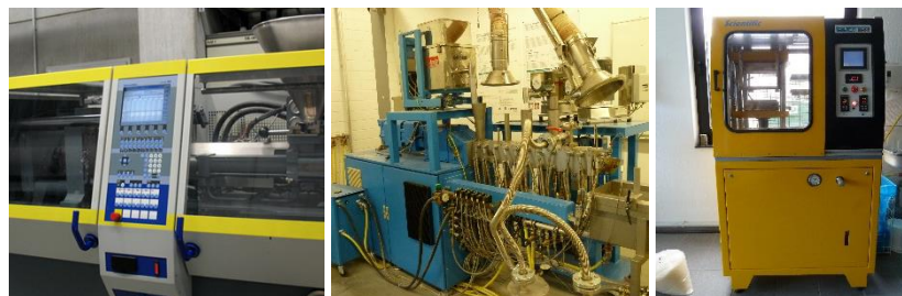
Figure 11: Machines for plastics recycling and downcycling; injection moulding machine (l.), laborextruder (m.), sheet press (r.) (© R. Kopitzky/Fraunhofer UMSICHT)
